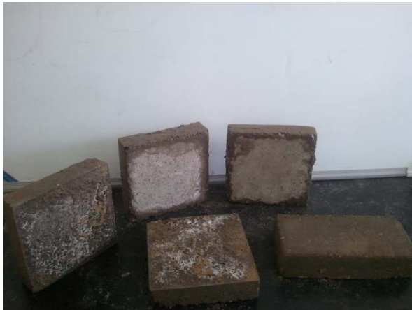
Figure 6: Geopolymer type concrete after keeping outside in winter condition
