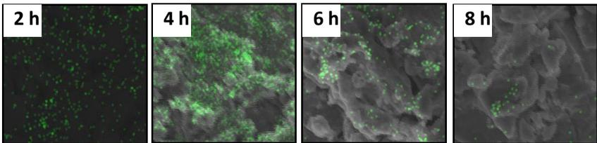
Fig. 2 SEM micrographs and the corresponding Mg element distributing of the  $\text{La}_{0.70}\text{Mg}_{0.3}\text{Ni}_{2.45}\text{Co}_{0.75}\text{Al}_{0.30}$  alloys annealed for different time
