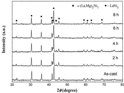
Fig. 1 XRD patterns of the as-cast  $\text{La}_{0.70}\text{Ni}_{2.45}\text{Co}_{0.75}\text{Al}_{0.30}$  and  $\text{La}_{0.70}\text{Mg}_{0.3}\text{Ni}_{2.45}\text{Co}_{0.75}\text{Al}_{0.30}$  alloys
