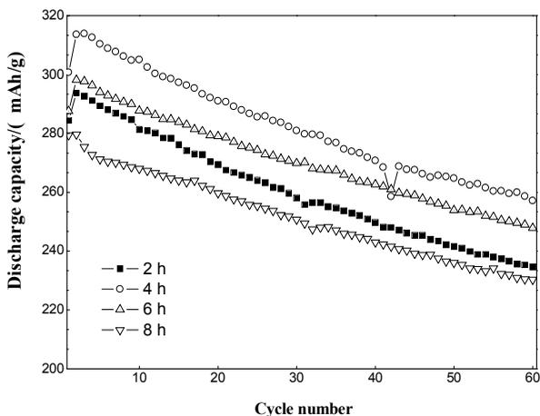
Fig. 3 Variations of discharge capacity with cycle number for the  $\text{La}_{0.70}\text{Mg}_{0.3}\text{Ni}_{2.45}\text{Co}_{0.75}\text{Al}_{0.30}$  alloys
