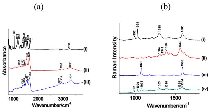
Fig. 2. (a) ATR spectra of solid (i) IMT and (ii) Tf. (iii) Infrared spectra of AuNP-IMT/TOPO-CBT-Tf in the wavenumber region between 800 and 3800  $\text{cm}^{-1}$ . The infrared TOPO spectrum[16] was omitted due to the weakness in comparison with the other IMT and Tf bands. (b) Raman spectra of (i) IMT and (ii) TOPO on AuNPs. SERS spectra of (iii) CBT and (iv) of AuNP-IMT/TOPO-CBT-Tf in the wavenumber region between 800 and 1800  $\text{cm}^{-1}$
