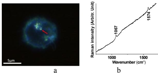
Fig. 4. DFM and SERS spectra of AuNP–IMT/TOPO–CBT–Tf embedded in a K562 cell. The arrows indicates the location of the AuNPs as determined according to the SERS spectra. The CBT-coated AuNPs were found to locate approximately a few mm inside the cell surfaces at the spot pointed by the arrows.
