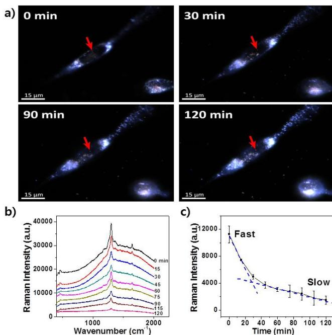
Fig. 6. (a) Photographs of the time-dependent in vitro dark-field microscopy (DFM) of live cell images. The arrows indicate the location of the AuNPs according to the SERS spectra. (b) Time-dependent SERRS spectra of MTX-conjugated AuNPs exhibiting the release of MTX. (c) Intensity of the SERRS spectra of MTX-AuNPs determined by measuring the intensities of the MTX peak at  $1291 \text{ cm}^{-1}$ . The standard deviations were obtained from independent measurements of three different cells
