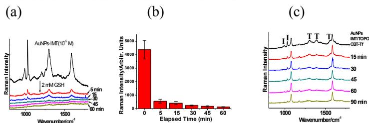
Fig. 3. (a) Release of IMT from AuNPs by GSH (2 mM) with an hour. The decrease in the SERS intensities of IMT indicated the desorption of IMT on AuNPs via GSH. Similar tests were performed for TOPO.[16] (b) Plot of the relative intensity ratios of the IMT band at 1030  $\text{cm}^{-1}$  after treating GSH (2 mM) for 0–60 min. (c) SERS spectra of AuNP–IMT/TOPO–CBT–Tf after treating with GSH. ‘I’ and ‘T’ stand for IMT and TOPO peaks, respectively
